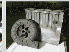
132T Rare 1933 Miller Block and Supercharger Casting
