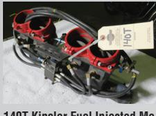
140T Kinsler Fuel Injected Mechanical 2 inch Manifold for Formula 1 or Vintage Midget
