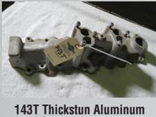
143T Thickstun Aluminum Dual Carb intake Flathead Speed Parts
