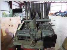
123T Reverse Flathead V8 60hp Motor with Offenhauser Heads for Midget Race Car Exhaust AND Intakes switched
