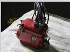
198T 4 Cylinder Midget Racing Magneto
