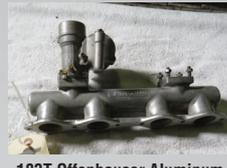
183T Offenhauser Aluminum Intake with dual Carbs-Only 1 Carb attached
