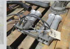
113T Vintage Aluminum Intake 4 Cylinder with Velocity Stacks
